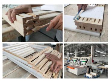
Door frame gluing process.
