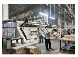
We utilize CNHF assembly machines to assemble doors and front frames. This machine dries the glue quickly, ensuring a strong and stable base structure.
