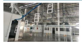
Paint coating line includes the primer and topcoat hanging line. After the paint is applied, the frames are sent to packaging. **Door Panel Processing**
