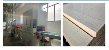
Parts are UV roller coated on both sides and then assembled.
