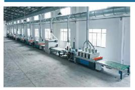
The panel is automatically roller coated. The white UV primer is perfected through automated color concentration.
