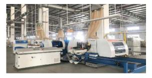
The double-end drilling machine from the Italian company, FRIULMAC processes door and frame parts, ensuring accuracy. FRIULMAC is internationally known as the technological leader in the woodworking sector.
