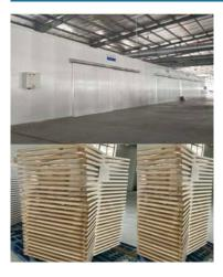
We let the frames dry for up to 48 hours. Frames are then sanded, drilled, and further prepped for assembly.
