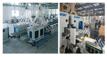
Our Double Sanding Milling Machine comes from the Taiwanese company HPOINT, and allows us to produce door panel parts within a tolerance of 0.1 mm.
