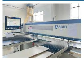
After UV processing, the cabinet will go through cutting process with each piece cut according to specification.
