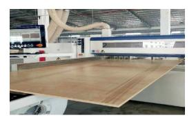
The cabinet boxes are cut according to the specification.
