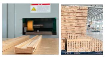
The raw material needs to be processed by a foursided molder machine to complete the frame parts as shown.
