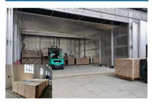
We are one of the few manufacturers in Vietnam to have our own drying kilns. Our four automated kilns have a capacity of 80 cubic meters each, ensuring a regulated moisture content.
