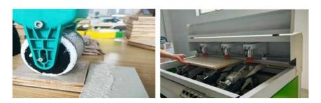
This stage includes cutting, gluing, cold pressing, edge banding, and drilling.
