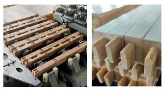
The final processing stages include milling, drilling, and tenoning.
