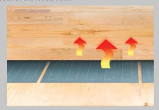
Since the heating mat with thermal cut-off is being installed at the same time as the floor it eliminates pre-running the system. Preheat the room to 10° F below desired room heat. Set floor thermostat to 5° F above its current temperature, and increase 5° F daily, until desired thermal comfort is achieved.
