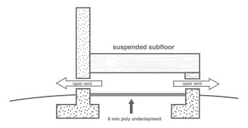
Size of available vents should equal to 1.5% of the square footage within the crawl space. Relative humidity should be consistent with interior of home. Moisture content of sub floor should not vary more than a 4% MC from the top of the sub floor to the bottom.
