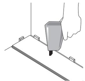
when the blind nail gun is too close to the wall to fasten down the planks.
