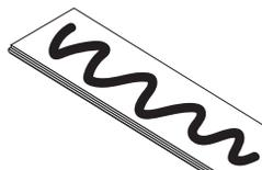
NOTE: Glue assist applications will not perform properly when applied to the surface of a vapor barrier such as Aquabar or 15lb roofing felt. Glue assist will only work on the wood subfloor itself without a vapor barrier applied.
