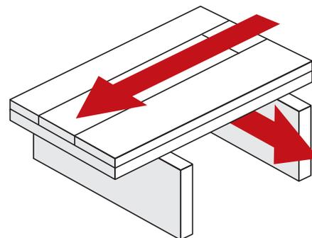
Additionally, nail (ring shank) or staple layers together on a minimum 12" grid pattern. Sheets should be glued to lumber subfloor using good quality
