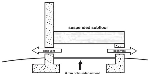
Size of available vents should equal to 1.5% of the square footage within the crawl space. Relative humidity should be consistent with interior of home.
