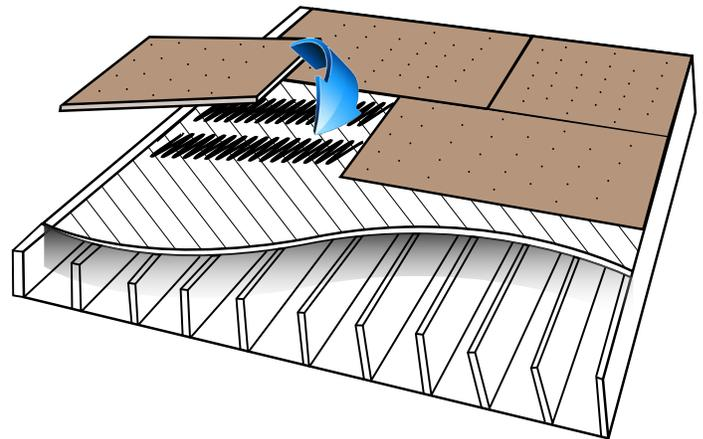
**NOTE: Do not install in the same direction as existing floor.**
