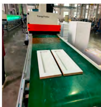
STEP 4: UV ROLLER BASE COATING
