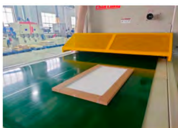
STEP 2: PRE-STAINING INSIDE EDGE OF DOOR FRAMES & CENTER PANELS TO ENSURE PROPER COVERAGE
