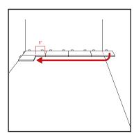
Use end cut piece from first row to start the second row. End joint spacing must be no less than 8" apart from rows on either side. Repeat process throughout the floor. Watch carefully to avoid lining up too many of the end joints and setting an obvious pattern.
