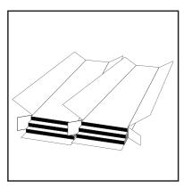
Always work from multiple boxes simultaneously and blend the planks throughout the installation. This is especially important in the event of multiple production dates.
