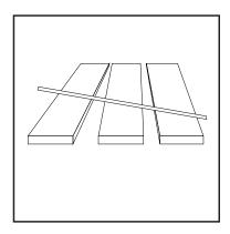
Before you get started, open multiple boxes and check how the planks / tiles blend with the moldings. At beginning of installation, set aside those planks that best blend to the transition moldings on job.
