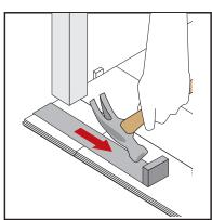
Ensure end joint at end last plank of the row is completely engaged with a pull tool.
