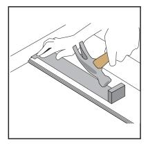
After engaging the side joints in the last row, slightly lift the edge of the plank. Using a pull tool, pull the plank completely into place. Follow up the length of the plank a second time and tap to ensure the joint is completely locked.
