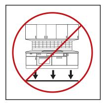
Installation of built in cabinets inhibits the ability for the floor to expand and contract. Perimeter gluing is also not recommended for the same reason.
