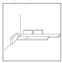
Standard expansion space should be factored at ¼" and this will suffice for a floor that does not exceed 50' in span or width.
