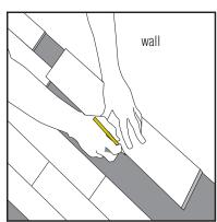
The last row of planks may need to be cut widthwise to achieve the correct width. The width of the last row must not be less than 2". This is accomplished by measuring the room prior to installation and factoring how many rows it will take to complete room.
