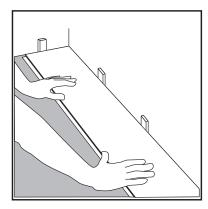
Select the longest wall in the room and install left to right, starting in the left-hand corner. For starting row, use adjustable spacers against side and end walls to maintain ¼" minimum expansion space. Use spacers at both the side and the end of the rows.
