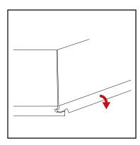
Insert short tongue end of the plank into groove at an angle and drop into place. Continue the process for the remainder of first row.
