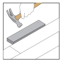
Use a tapping block and hammer, tap the block against the plank edge to fully engage the locking system. Failure to fully engage the locking system will cause the joints to open up later. CAUTION: Do not strike the edge of the plank or the locking system with the hammer.
