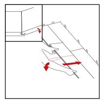
At a slight angle, insert tongue end into the grove end of the previous plank. Get as close to the side of the previous plank as possible. Also at a slight angle, press the side tongue into the groove of the plank next to it. Press gently to engage the planks.
