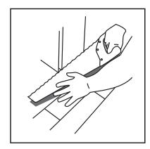
Remove all shoe and base molding to ensure adequate expansion space. Use scrap piece of flooring to establish height of cut.
