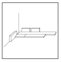
For starting row, cut blocks to use against side and end walls to maintain ¼" minimum expansion space. Use spacers at both side the end of the rows. Use of adjustable spacers may be needed to help maintain a straight edge line, if not scribing the floor.
