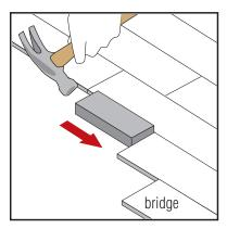
Using a tapping block and hammer, tap the end of the plank edge with the block to ensure that the locking mechanism is fully engaged. Do not strike the edge of the plank or locking mechanism with the hammer. If edges are unsightly, and the joint could be compromised.
