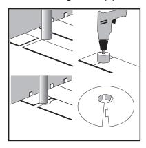
If the room has pipes or radiators or pipes, drill a hole large enough to fit around them with space for expansion.
