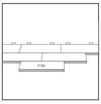
Using a cut piece of approximately 12" to 14" in length, form a temporary bridge next to the end of the plank just installed.
