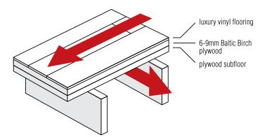
6. Sub floor Prep: OSB & Sub floor Rated Plywood are acceptable for use under Hallmark Floating/Locking. All nails must be countersunk, all panel edges must be sanded flat. Sub floor joints must be feather filled with a Portland based patch and allowed to dry.
