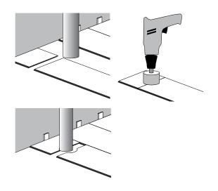
2. Wrap the pipe with a radiator pipe collar to cover expansion space. Plastic collars are available at home improvement stores and plumbing supply stores. Wood collars are specialized and can be located at some hardwood flooring distributors, or specialized wood websites.
